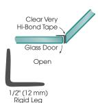
This Clear Polycarbonate Angle Jamb is used for both hinge and strike jambs. It can be adhered to the wall or a fixed panel using our Clear Very Hi-Bond Tape.
